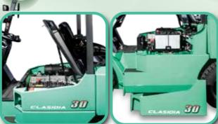
The new Clasidia was designed so that troubleshooting and repairs are easy and require no specialized tools. Access to the engine bay is as simple as pushing a small button and lifting up engine cover. The engine bay is well laid out and there is plenty of room to carry out routine maintenance, service or repairs.
