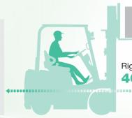
Right angle stacking aisle width 4085 mm • FD25HS
