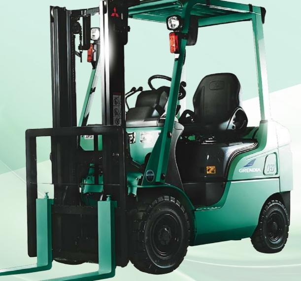
Electronically controlled gasoline engine Capacity rating 1500kg @ 500mm load center
