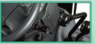
**Combination switch** integrating indicators and headlight switches.
